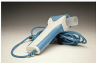
USB-based spirometer with software integration for the AFHCAN software.
