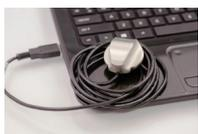
USB-based stethoscope with live teleauscultation software. Used in conjunction with Vidyo-based videoconferencing.
