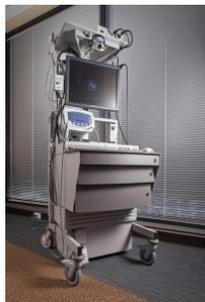
AFHCAN V4 Cart without biomedical peripherals. This cart includes the monitor, scanner, keyboard, mouse, 115v hospital grade power supply system.
