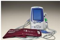
USB-based vital signs monitor with attachments for: blood pressure, pulse, pulse oximetry, and temperature.
