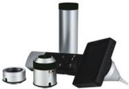
A multipurpose examination camera with otoscope, dermascope, and general exam lenses. Has built-in USB 2.0 and can be used as a live video input for AFHCAN and Vidyo, or as a stand-alone digital camera with microSD storage.
