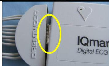
**4.** May try gently wiping lead ends with dry gauze and friction in case of possible corrosion.
