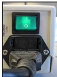
2. Turn on the video otoscope light source by pressing the green POWER button. The standby light will go out.
